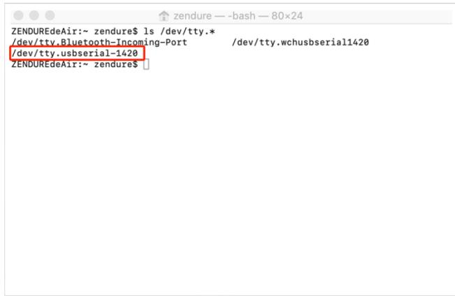
A screenshot of a terminal window titled "zendure — bash — 80x24". The command "ls /dev/tty.\*" has been entered and is being processed. The output shows several device files, including "/dev/tty.Bluetooth-Incoming-Port", "/dev/tty.usbserial-1420", and "/dev/tty.wchusbserial1420". The line containing "/dev/tty.usbserial-1420" is highlighted with a red rectangle. The window shows three gray dots at the top left, indicating it is still running.
